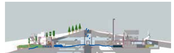
Rain onto chapel floor center drains left to the Living Machine at the Lodge grotto then right to the cistern below the music store at the Arena. Vented dampness controls keep instruments above from drying and cracking.
